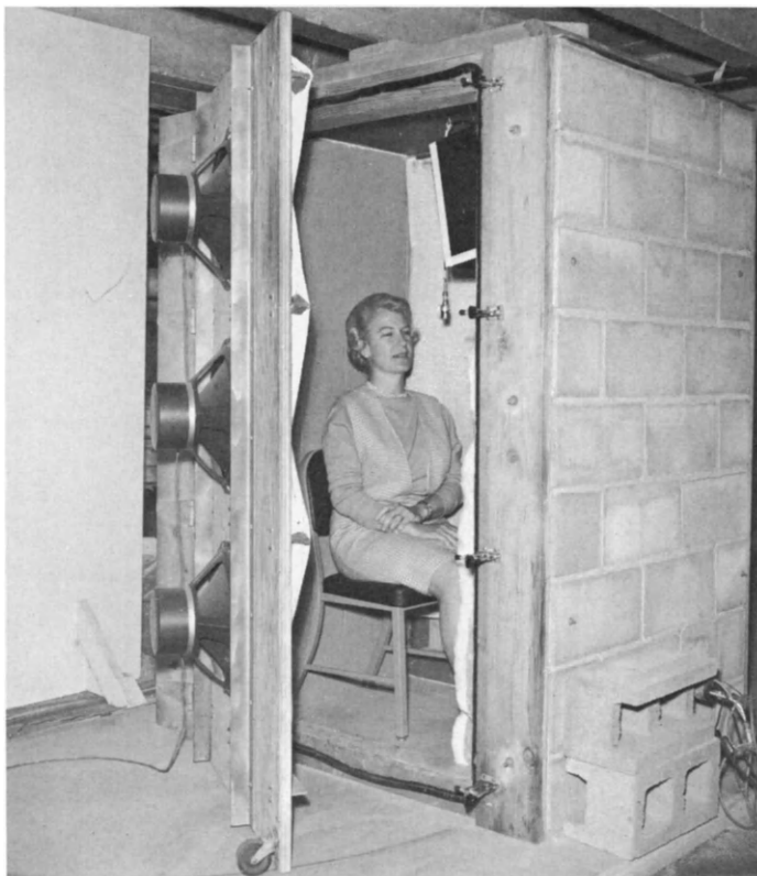
FIGURE 228. Sonic boom simulation chamber. Note hinged wall access. From Shepherd and Sutherland (735).
